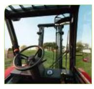
Optional fully enclosed cab with heater, defroster and air conditioning.
